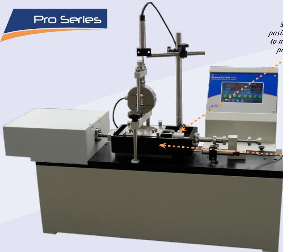
*Submersible load cell positioned in the water bath to measure load as close as possible to the sample.*
