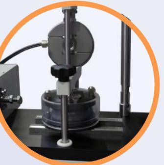
*Water carriage removed and Consolidation Cell placed on adaptor, ready for Oedometer testing*
